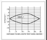
APPLICATION NOTE: as a general rule regarding background objects in diffuse sensing, verify that the distance to the nearest background object is at least three times the distance from the sensor to the object to be sensed. For example, if a product passes one inch from an SBD1 sensor, the nearest background object should be at least three inches further away.
